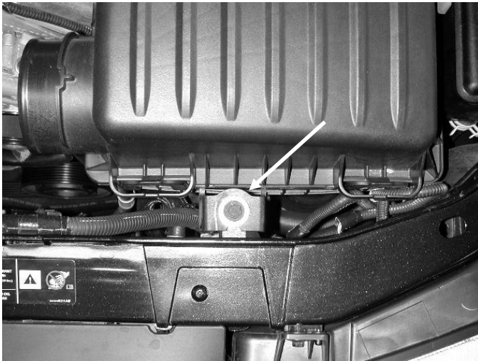
g) Loosen and remove mounting bolt. This bolt will be reused.
