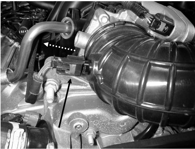
c) Pull out the locking clip for the I ntake A ir T emperature sensor.
