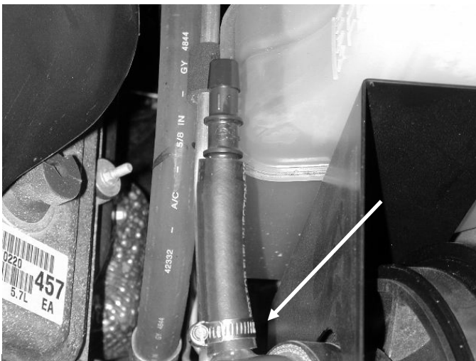
r) Tighten the breather hose to the nipple with the provided hose clamp. Please make sure to trim the hose length for best routing if the 2009 MY and up adapter is installed (refer to step q).
