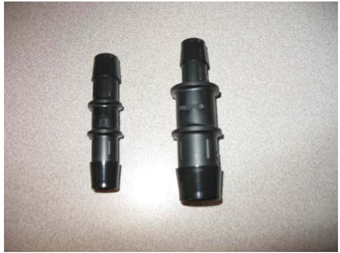
q) Insert supplied connector into the breather hose. For 2009 model year and up, use the reducer adapter shown on the right. For pre-2009 model year vehicles use the straight adapter shown on the left. Use lubrication as necessary.
