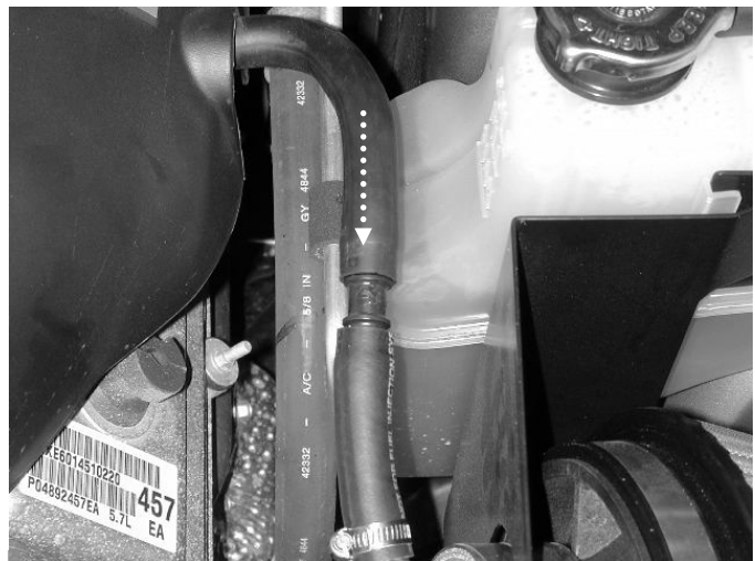
s) Attach the factory breather hose to the connector.
